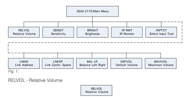
Relative volume for the active input. Fine tuning of the volume control for each input relative to the global setting. The Sensitivity can be adjusted +/-6dB in 0.1 dB steps.
